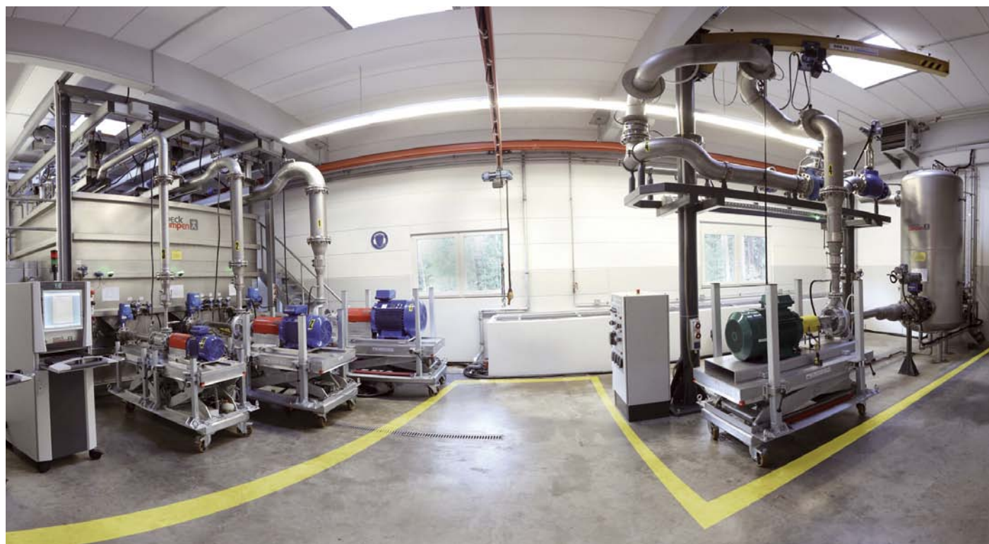
Computer-controlled and fully automated test stands on the premises of Speck in Roth. Measuring of hydraulics, power requirements, axial thrust, vibrations and NPSH values. Heads of up to 400 m and flow rates of up to 750 m 3 /h are possible..
